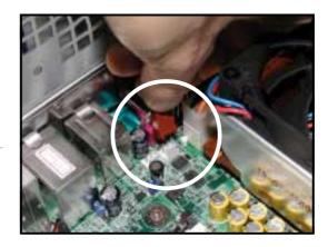
Make sure that the heatsink and fan assembly is stable in place and the fan power cable plug is properly connected.
